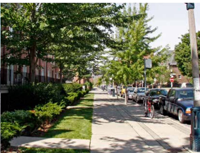
Differentiate pedestrian throughzones from the furnishings zone through different paving treatments
