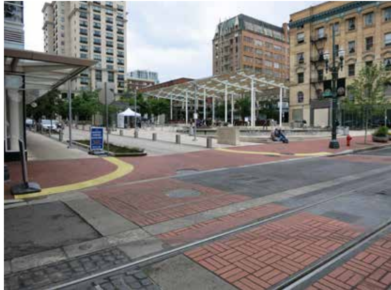
Clear markings and reduced turning radii can enhance pedestrian safety at intersections
