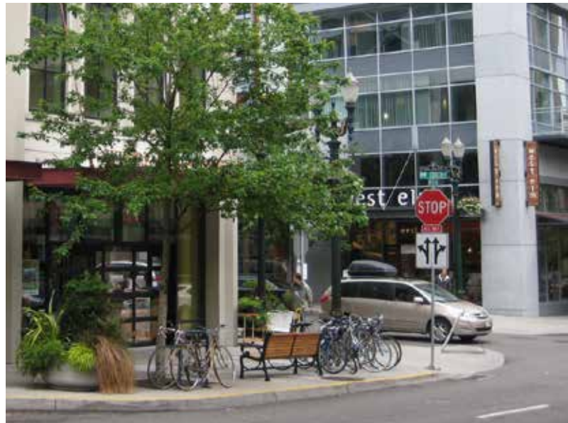
Bump-outs and reduced corner radii shorten crossing distances and create additional sidewalk space for pedestrian and cycling amenities
