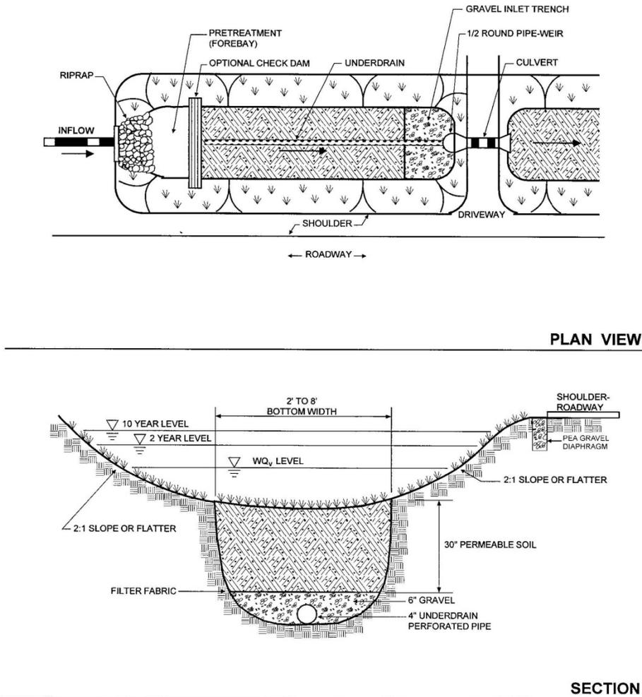
Figure 28. Bioswale typical plan and cross-section. Source: NYS Stormwater Manual
