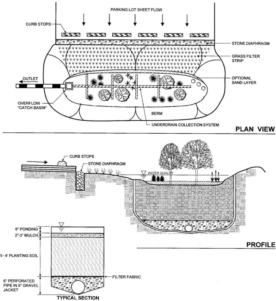
Figure 35. Biofilter typical plan and cross-section. *Source: NYS Stormwater Manual*
