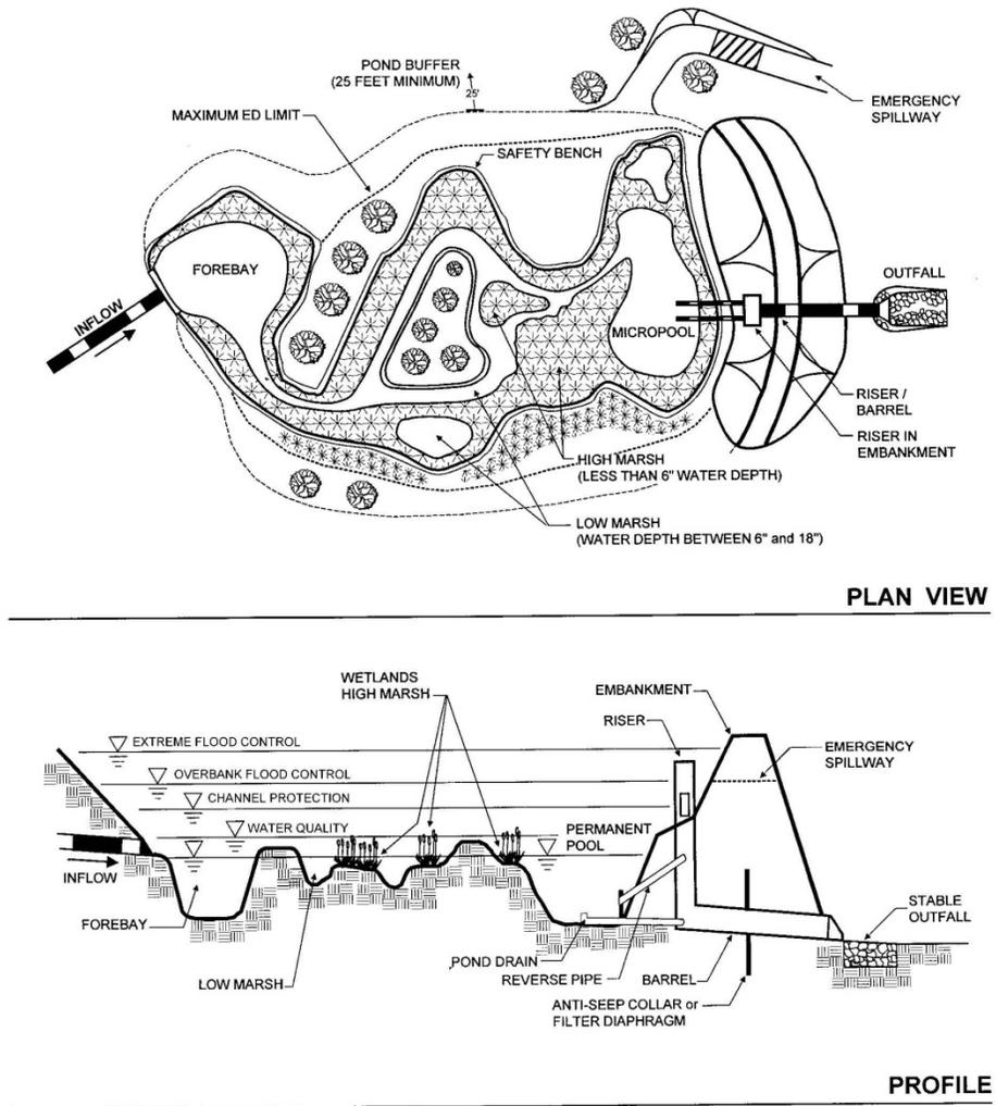
Figure 42. Stormwater wetland typical plan and cross-section. Source: NYS Stormwater Manual
