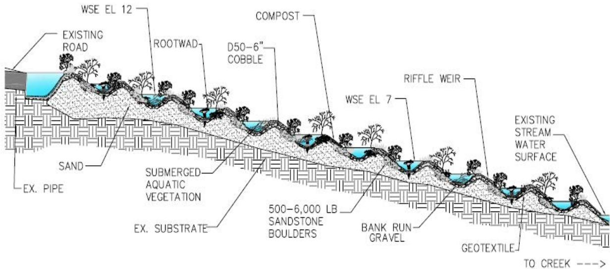
Figure 45. RSC typical cross-section. *Credit Biohabitats*
