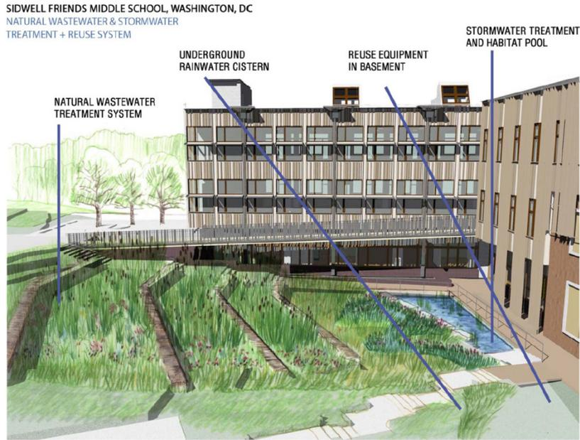
Figure 46. Constructed treatment wetlands are integrated into the design of the landscape at the Sidwell Friends School in Washington, DC. *Copyright NSI*
